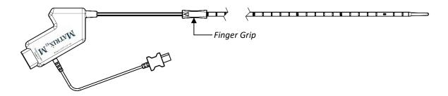
(d) Once probe is placed, grasp probe's connector housing with one hand and grasp finger grip with the other hand. Keeping probe in place, pull back until finger grip is seated on housing.
